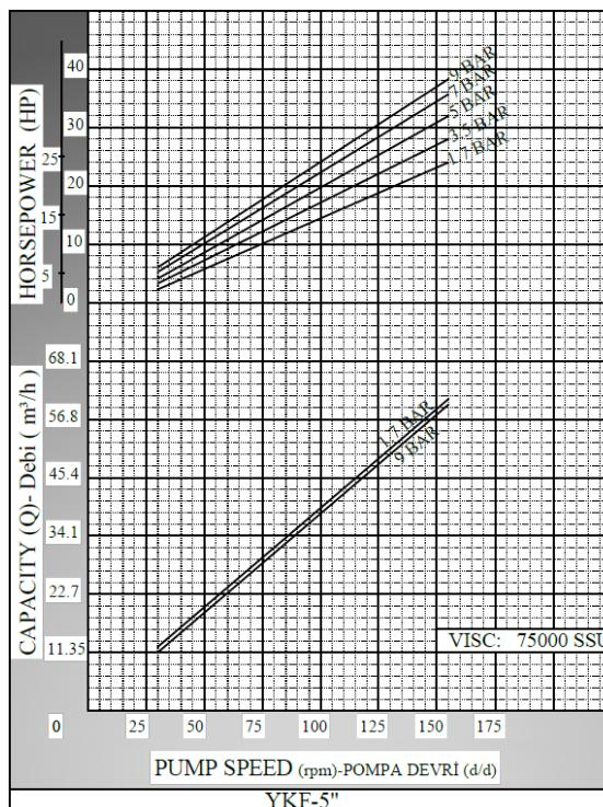
PUMP SPEED (rpm)-POMPA DEVRI (d/d)
