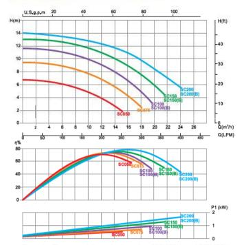
Remarks: Flow curve information based on 220V/50Hz and 380V/50Hz motor.
