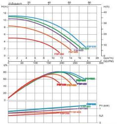
Remarks: Flow curve information based on 220V/50Hz motor.
